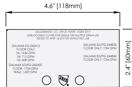
SPECIFICATION PLATE DETAIL
